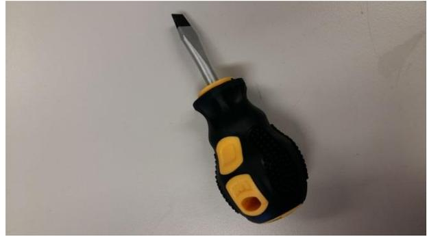
Figure 7: Flat-head screw driver for adjusting the beam size of the laser diode
