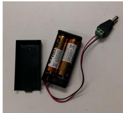
Figure 3: Battery pack with 2×1.5V AA batteries and outlet plug for the laser diode
